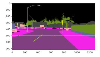
*Figure 2.* Determining left and right distances for feature extraction. The green and red markers represent the road boundaries and their distance respectively from the left and right edges of the frame is computed and normalized using the respective left and right distances of the blue and orange markers.
